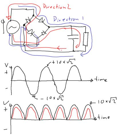
5 marks for the correct bridge rectifier, with arrows.3 marks for correct input/output waveform, with magnitudes.2 marks for the diode losses (red line).
