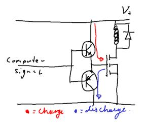
3 marks for the diagram. Deduct 1 mark for each mistake.2 marks for: The use of the push pull pair enables fast charging/discharging of the MOSFET.
